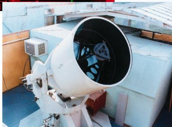
Working as regular laser ranging station of satellite. Measuring the distances to satellite till 20000 km with accuracy about 1 cm or lower.
