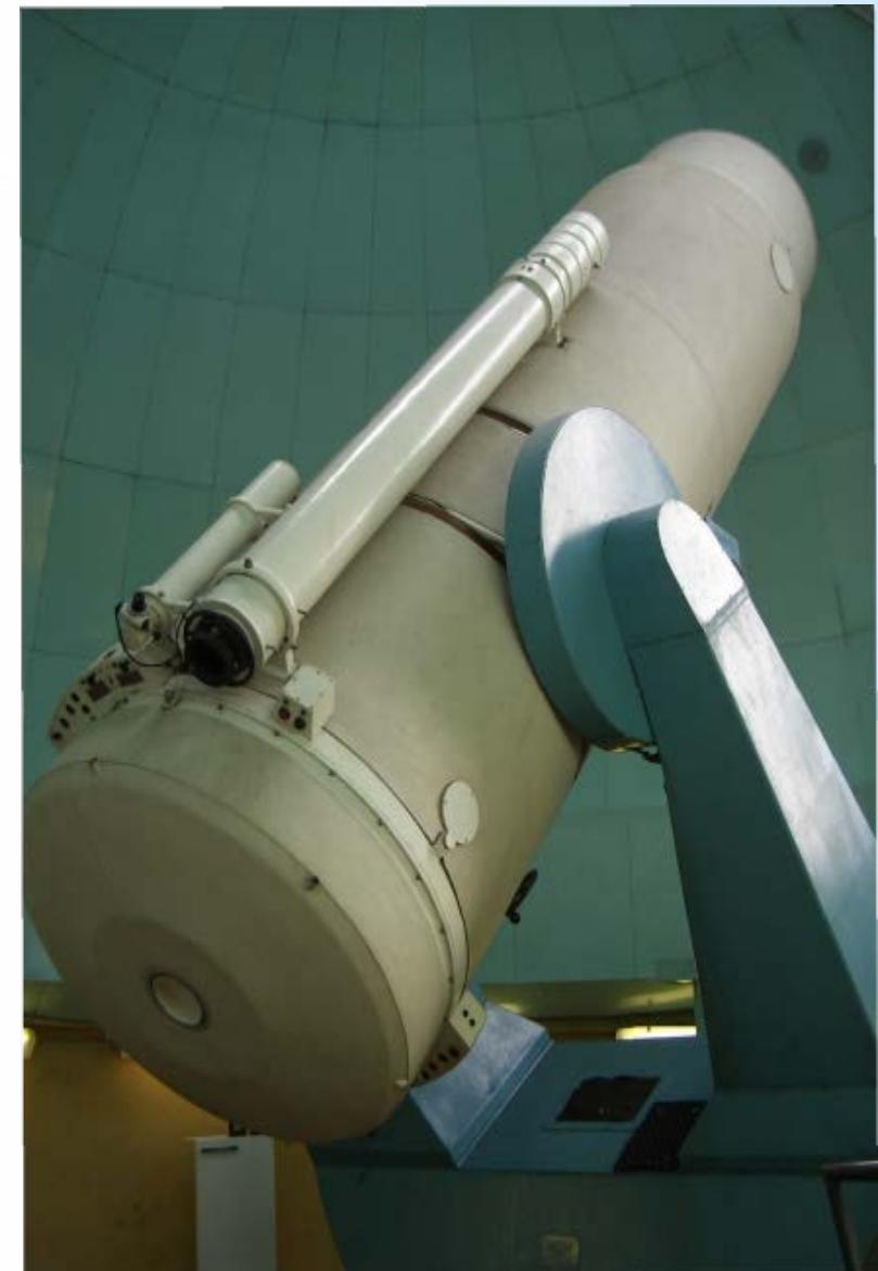
Baldone Schmidt type telescope main mirror 1,2 m, entrance aperture 80 cm, focal length 240 cm. Coated in 2006 and installed by 3,2MB CCD. 4 degree objective prism, spectral resolution 500.
